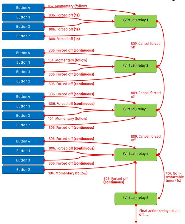
To avoid the LEDs giving away the sequence, it is advisable to set the LED feedback of the buttons to "Monitoring" (in the configuration settings of the input module, tab "LED feedback"). The monitored channel can be virtual relay 5 (in that case the LEDs on the buttons will light up for 1 sec. when the correct sequence has been completed), or no monitoring action at all can be used, in which case the LEDs will simply remain off.
