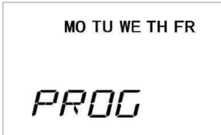
Press BOOST/OK to enter the group programming mode. The thermostat displays the first switching point (P1). Note that the time of this switching point cannot be modified.
