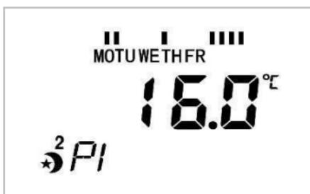
Press BOOST/OK to confirm. Now, select the switching point time with the dial. Press BOOST/OK to confirm and to enter the second switching point (P2).
