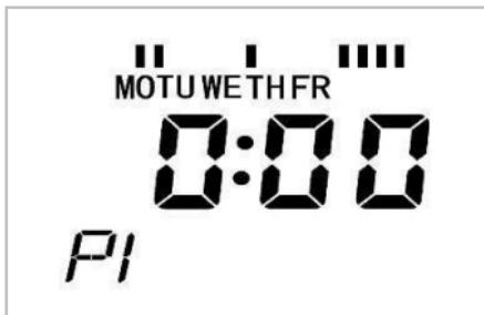
Press BOOST/OK to confirm. Now, select the temperature mode with the dial.
