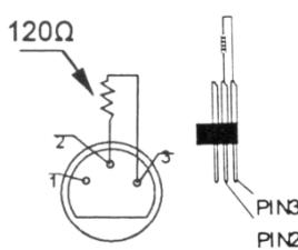
A DMX terminator is recommended for installations where the DMX cable has to run a long distance or is in an electrically noisy environment (e.g. discos). The terminator prevents corruption of the digital control signal by electrical noise. The DMX terminator is simply an XLR plug with a 120Ω resistor between pins 2 and 3, which is then plugged into the XLR output socket of the last device in the chain.
