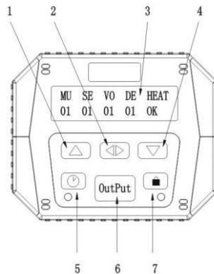
Plug the remote control into the rear of the smoke machine. Once the smoke machine is connected to the mains and switched on, the main switch will light indicating the unit is receiving power. The bar beneath the HEAT indication on the remote control display will blink. After a warm-up time of  $\pm$  5 minutes, the blinking bar will switch to OK, indicating the unit is ready.
