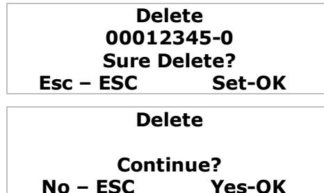
Press OK to delete, and press ESC to exit, if a registration number has backup passwords, the screen will be prompted to delete backup data.
