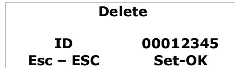
Use the number keys to input the Registered No (User ID No.) which has to be deleted from the machine, e.g. 12345, as follow:
