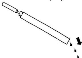
5. Remove the cooling strip with a pair of pliers.
