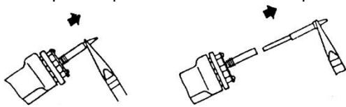
6. Reinsert the stainless tube in the heating element to melt the solder. This takes approximately 5 seconds.
