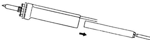
4. Point the collector down and shake it gently so that the waste solder falls out. Do this frequently to keep the station in proper working order.
