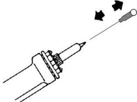
4. Unscrew the barrel nut assembly.
