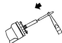
7. Remove the stainless tube and shake loose the molten solder.
