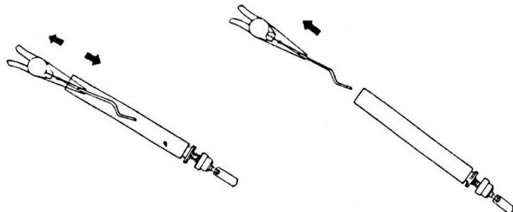
6. Clean the cooling strip and collector with a wire brush (included).
