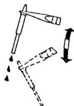
8. Check if the tip is unclogged, then put it back in place and screw down the barrel nut assembly. Do not over-tighten.
