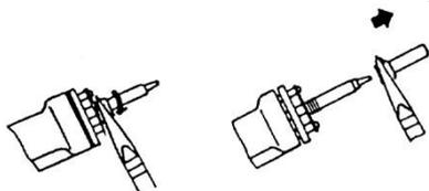
5. Use a pair of pliers to remove the tip.
