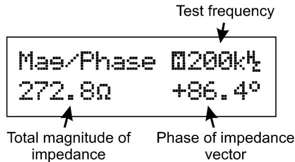
This display is useful for gauging how close your component is to a theoretical “ideal” inductor, capacitor or resistor.
