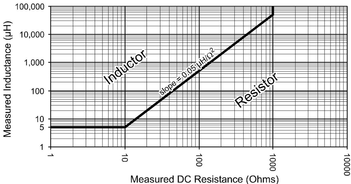
For example, if the inductance of your component is measured at  $100\mu\text{H}$  and it has a DC resistance of  $100\Omega$ , then the LCR45 will tell you that you have a resistor. If however the resistance was only  $10\Omega$ , then the LCR45 will tell you that you have an inductor.
