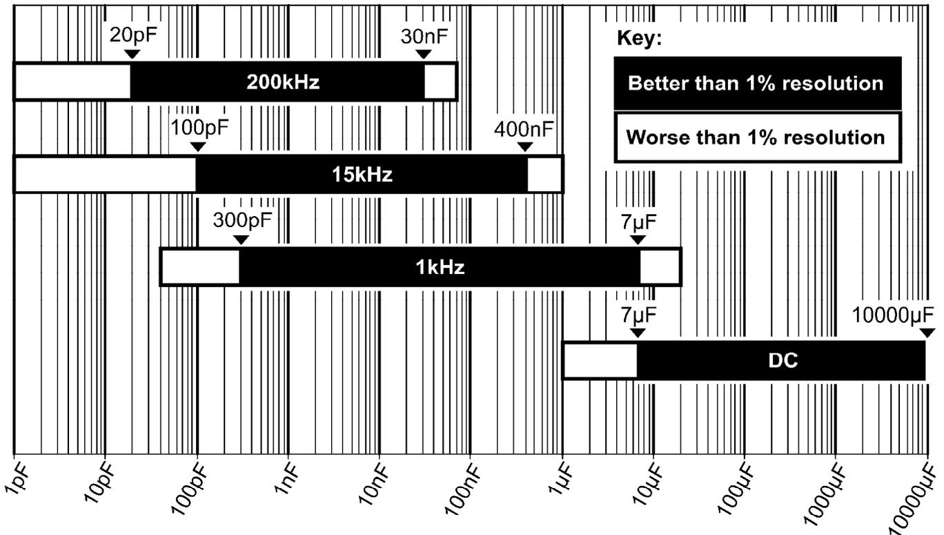
Measuring capacitance outside of the black bands will result in degraded measurement resolution (possibly worse than 1% of the measured value).
