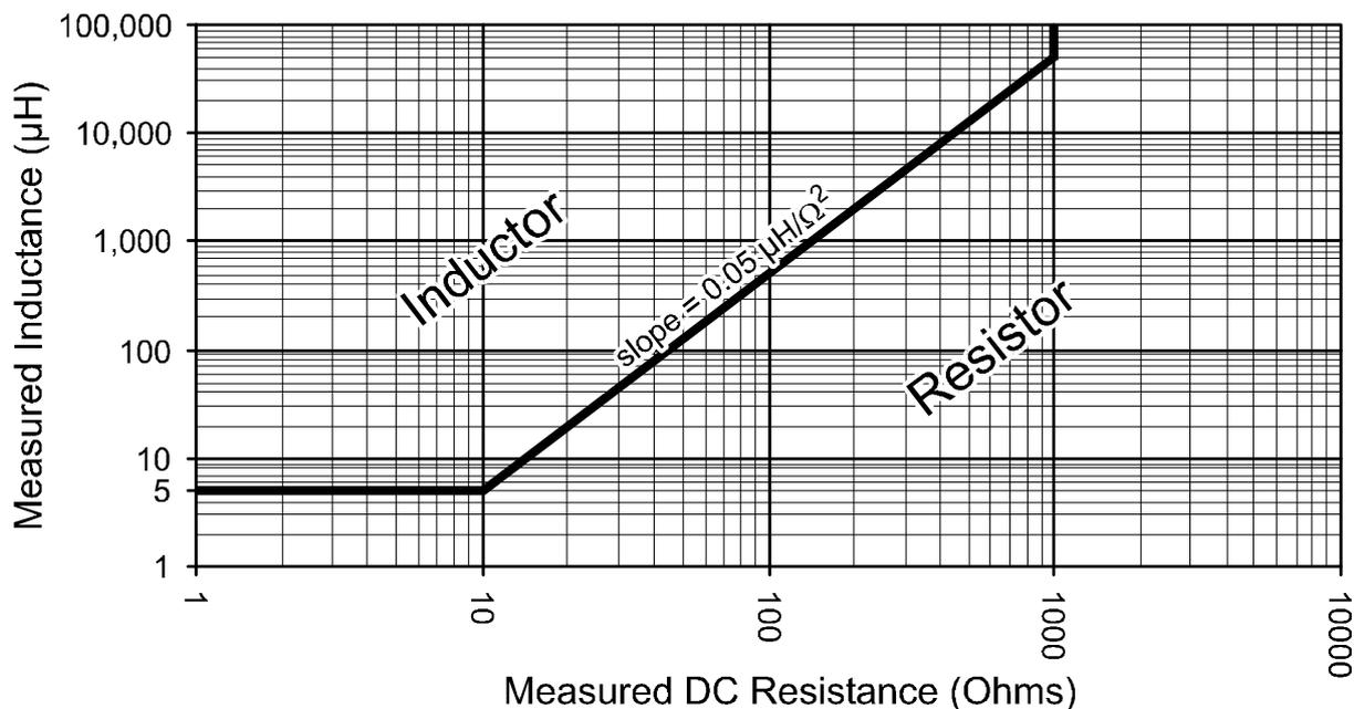
For example, if the inductance of your component is measured at  $100\mu\text{H}$  and it has a DC resistance of  $100\Omega$ , then the Atlas LCR will tell you that you have a resistor. If however the resistance was only  $10\Omega$ , then the Atlas LCR will tell you that you have an inductor.
