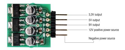
From the circuit diagram, it is possible to see that the three regulators are connected in a parallel configuration, that is to say that the input of each one of them is in parallel with the other ones; thus all three are powered by the voltage applied between the 12 V and GND (ground) contacts. All the contacts (inputs and outputs) are placed on the borders for an easier wiring, and are repeated on a line of spacing 2.54 mm bonding pads, that enables the assembling of a pin-strip.
