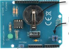
Back-up battery: provides power to the shield when the Arduino Uno is not active
