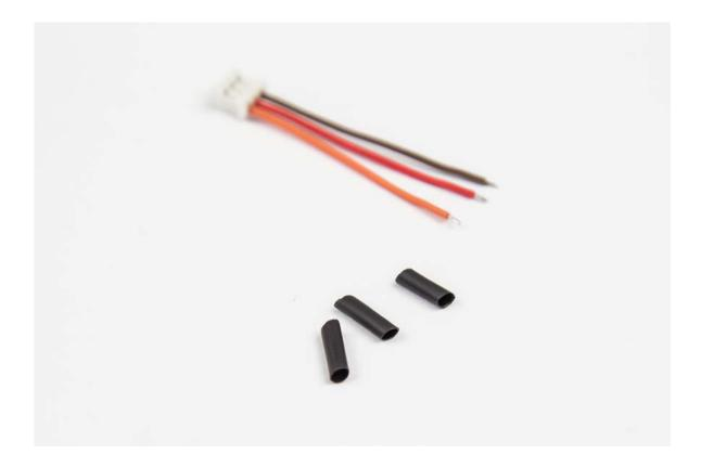
41. Solder the wires to the selector switch as shown below. **Do not forget the shrinktube pieces** and note the colors.
