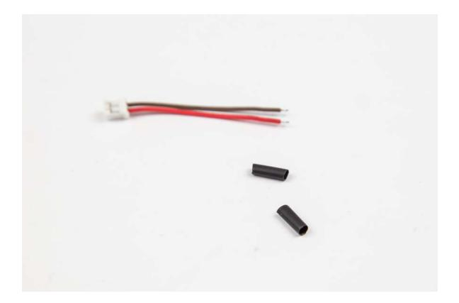
37. Solder the wires to the footswitch as shown below. **Do not forget the shrinktube pieces and note the colors.**
