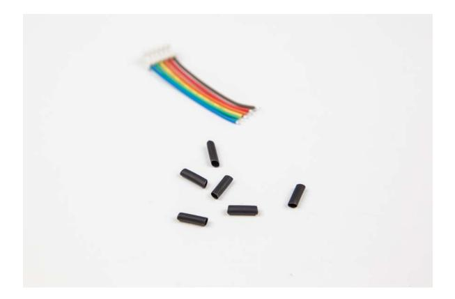
33. Solder the wires to the footswitch as shown below. **Do not forget the shrinktube pieces and note the colors.**
