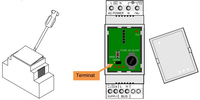
In normal circumstances only 2 'TERM' terminators must be foreseen in a complete Velbus installation. Usually this will be on one module inside the distribution box and on the module the furthest from the distribution box.
