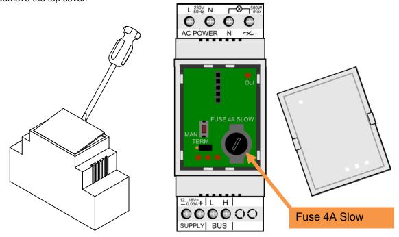
Use a screwdriver and slightly push the cap of the fuse holder down before unscrewing the fuse holder anticlockwise. Use a pair of long nose pliers to lift the cap. Replace the fuse and screw the cap back in place.
