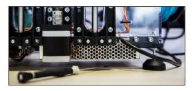
It is stated in the manual that additional protection might be needed depending on the user environment and operator skills. To prevent accidental contact in certain environments where the printer is operated by non-skilled persons a cover will be made available (code K8405). This cover will wrap the entire power supply and provides supplementary protection against accidental intrusion of small conductive materials.
