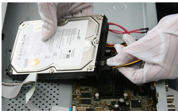
Figure 2-3 Connect Power Cable
