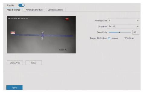
**Figure 5-10 Line Crossing Detection**
