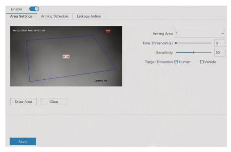
**Figure 5-11 Intrusion Detection**
