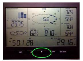
To tell the weather station to start communicating with the software, press and hold the button showing a down arrow until the weather station beeps (approximately 3-4 seconds).
