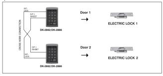
An inter-lock system needs two door controllers. This application example uses two keypads with simple cross wire connection on their "Output 1 Inhibit" and "Inter-lock Control Output" terminals. It is necessary to link up the "(-) GND" terminals of the two keypads as common ground to achieve the inter-lock logical functions.
