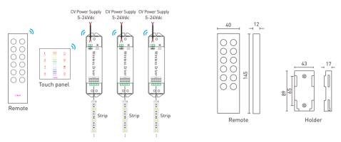
F series remote can control wireless driver directly, please refer to wireless driver manual for match code method.
