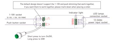
12V lamp connected, loads 0~144W(12V).
