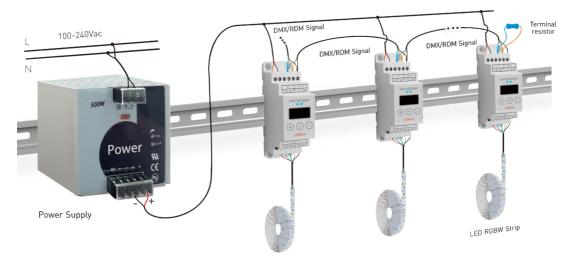
\* An amplifier is needed when more than 32 decoders are connected, signal amplification should not be more than 5 times continuously.
