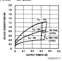
**Device Dissipation vs Output** Power —  $8\Omega$  Load
