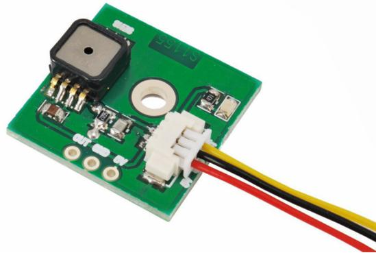
This is a 5V powered breakout board equipped with a pressure transducer, a component produced by Freescale and signed as MPXH6115A6U. This sensor provides an analog output signal, the reason why it may be used in order to directly pilot some small tools having pointers, and so to obtain immediate indications concerning the pressure that is being measured: for example, in a pipe in which air is flowing, or in a sealed container.
