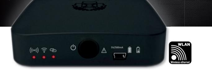
The Velleman WFS210 is the world's first wlan dual channel digital storage oscilloscope geared towards tablet computers. The WFS210 is a compact, portable battery powered fully featured two channel oscilloscope. Instead of a built-in screen it uses your tablet (iOS, Android<sup>™</sup> or PC(Windows)) to display the measurements. Data exchange between the tablet and the oscilloscope is via wlan.
